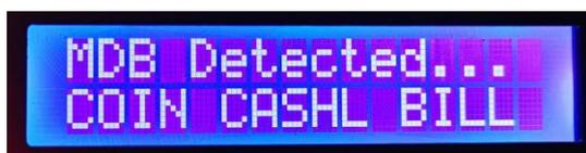
After finished the device detecting,then it enters the normal operation interface.Then it is possible to make payment through the payment device
